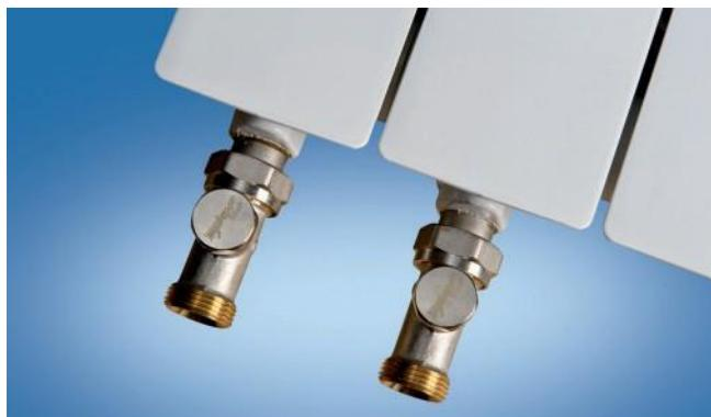
Each Orion+, Solar+ or Plano+ radiator comprises two appropriate radiator columns which have stop valves. The stop valves allow the radiators to be connected to or disconnected from the heating installation, and with the aid of the respective transitional piece, i.e. fitting, they can be connected to all types of "two-piping" installations.
